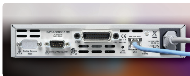
Figure 2. A modular LXI instrument uses the RJ-45 LAN connector (blue wire) to communicate with a PC controller through an existing LAN infrastructure.
